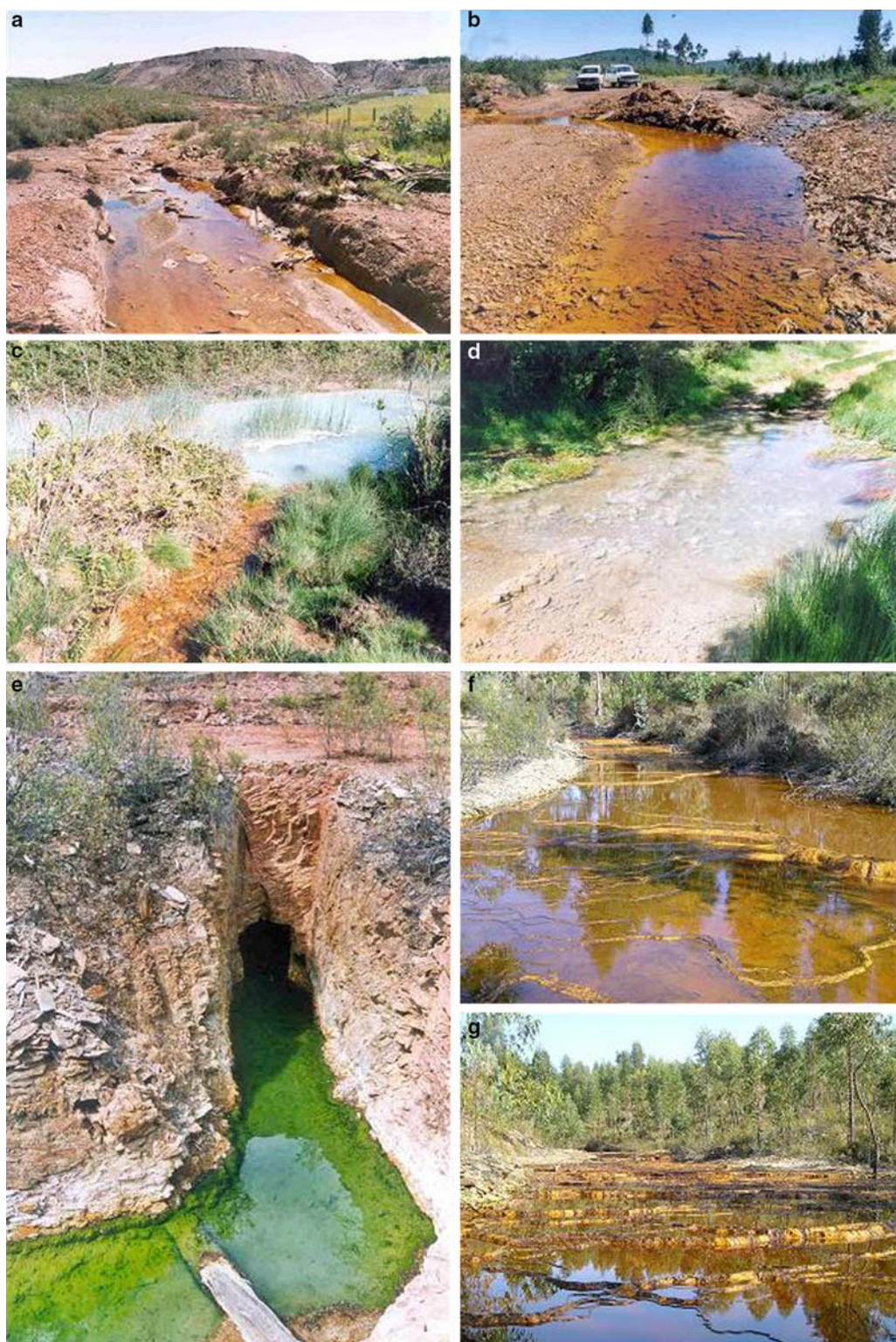
Fig. 3 Photographs of some sampling points in the studied effluents: a waste pile and acidic effluent in Tharsis as seen from sampling point DB-1; b confluence of two acidic effluents in DB-3 (Tharsis); c transition from Fe-precipitating (pH 3.1) to Al-precipitating (pH 4.3) aqueous acid solution between DB-7 and
